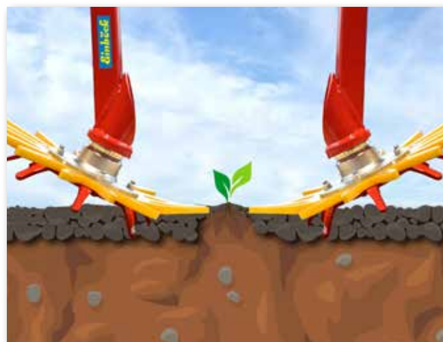
Equal working depth of both finger weeders due to common extension arm
