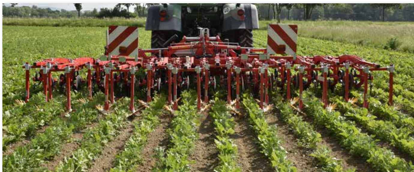
A preloaded spring ensures consistent working quality of the finger weeders
